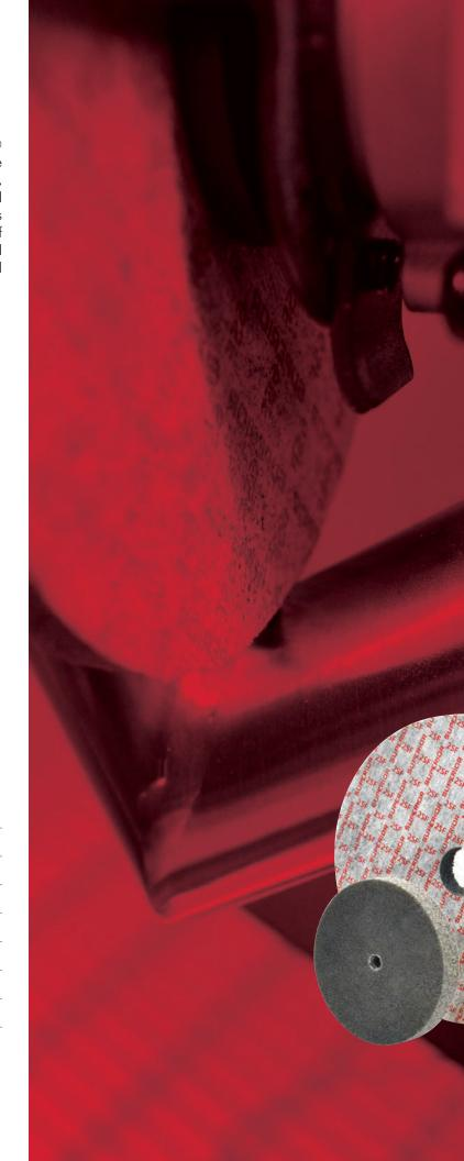
Layered sheets of nonwoven abrasives are compressed in resins, forming a dense slab, from which smaller diameter wheels are produced. The density of unitized wheels allows controlled cutting, cleaning and polishing action for tighter tolerances.
