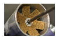
Flex shaft tools are used for extended depths or routing stars through curved tubing or pipe. Mandrel extensions are used well for boring & shaping, cleaning or deburring of tubes, drilled holes or cylindrical parts of moderate depth or slightly out of reach.
